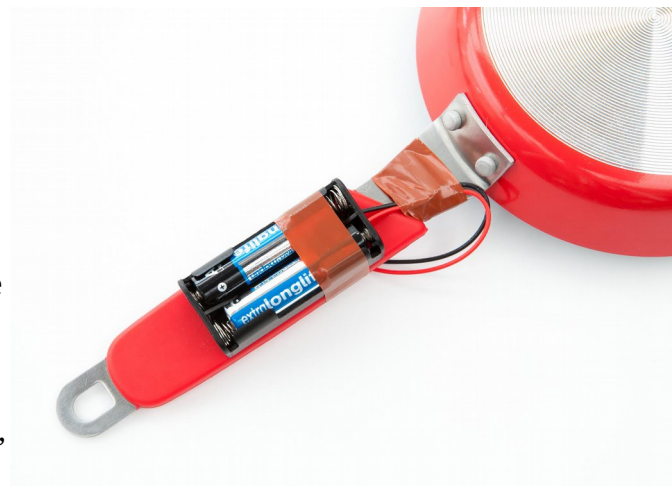
Figure 9: Fixing the battery pack with tape
