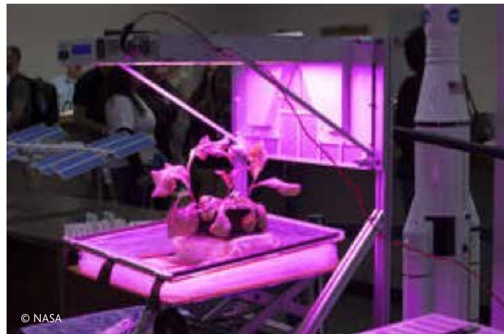
**Figure 2** The VEGGIE project explored ways of growing different plants in conditions similar to those found in space. The pink glow is caused by a combination of red and blue LEDs that provide the correct wavelengths of light for photosynthesis.
