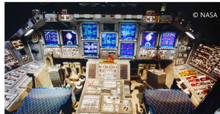
Figure 2 Shuttle flight deck, including 11 different screen displays
